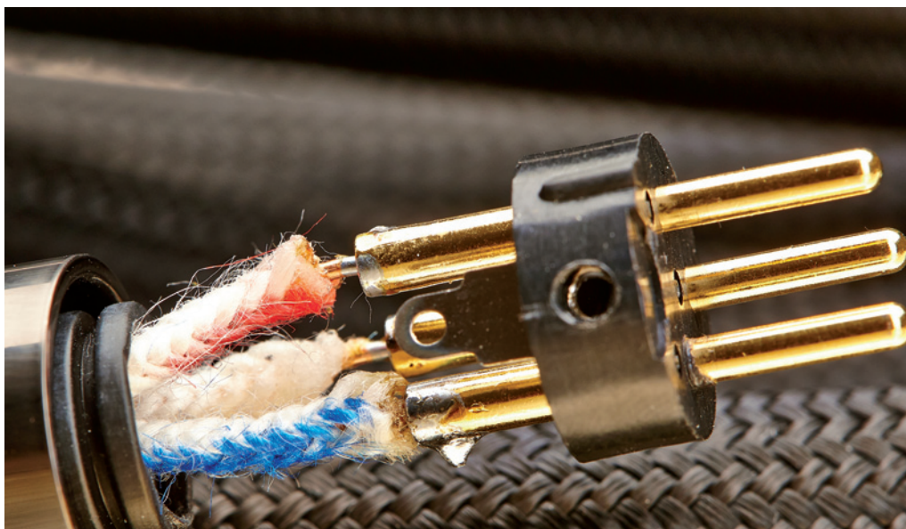
As seen here, no synthetic polymers are used as dielectrics
